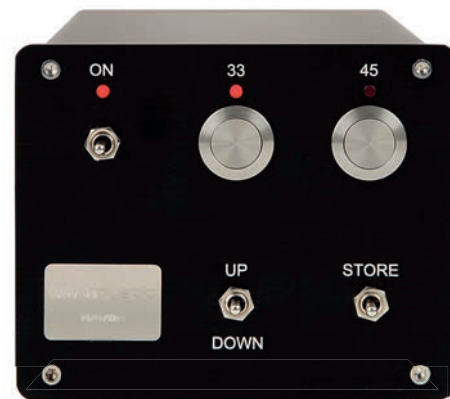
ABOVE: The DC power supply has incremental speed adjustment for 33.3 and 45rpm
