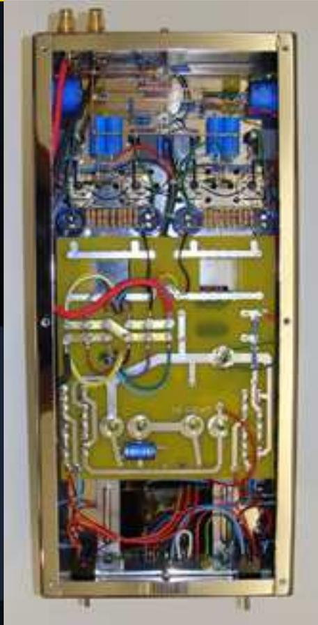
From the inside this model is an expression of all our savoir-faire in manufacturing, following all the rules of cabling of the army's radio communication systems. Components are connected in "3D" in order to avoid any electromagnetic interactions and disturbance. Only the power supply side is produced on printed circuit
