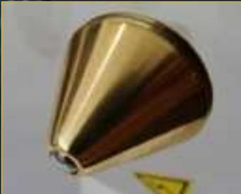
The apparel rests upon four feet with a conic shape. They are made with brass and a steel ball is set on the top. This process allows a minimum contact surface with the support and therefore the apparel is isolated from any vibrations.
