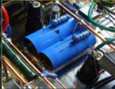
**Teflon technology linking capacitor.** This dielectric material is greatly appreciated because it allows the component benefiting from it to keep the passing signal untouched and insure at the same time a decisive musicality for the circuit using it.
